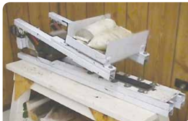
In the Schlulze Breuer Ruck test small "pills" prepared from the slurry ingredients in fixed proportions are subjected to water soak and abrasion, eventually in boiling water, and the damage assessed on a points scale
