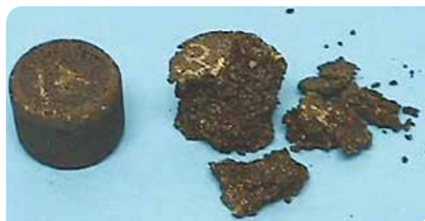
In the Schlulze Breuer Ruck test small "pills" prepared from the slurry ingredients in fixed proportions are subjected to water soak and abrasion, eventually in boiling water, and the damage assessed on a points scale
